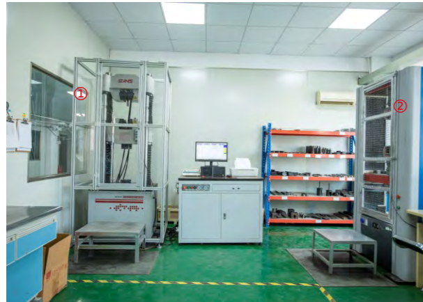
Microcomputer Controlled Electro-hydraulic Servo Universal Testing Machine Microcomputer Controlled Electronic Universal Testing Machine
