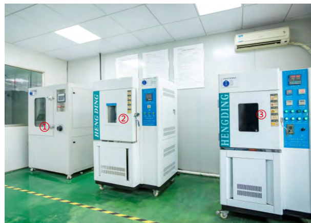
① Spray Electric trace Resistance Tester ② High & low Temperature Test Chamber ③ Xenon Lamp Aging Test Chamber
